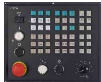
Control Panel for Mill
