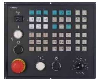
Control Panel for Mill
